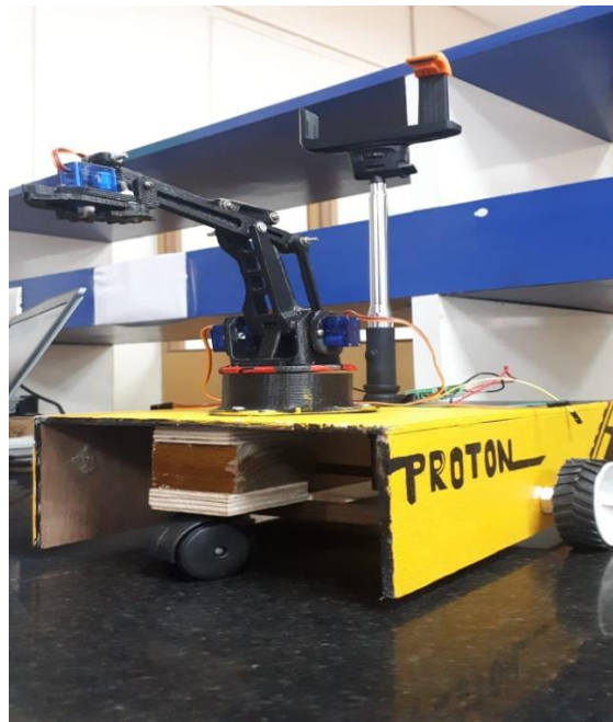
Fig 4. Image of the vehicular bot with an arm mounted on it.
